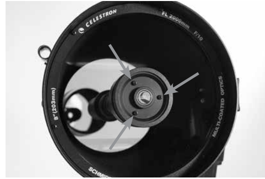
Secondary Mirror Collimation Adjustment Screws
